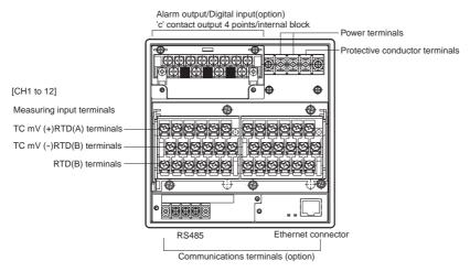
Alarm relay output (4 points 'c' contact)
