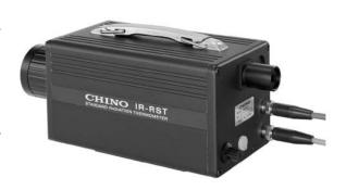
0.9µm model supplies JCSS\*\* calibration which certifies temperature range from 400 to 2000°C by fixed point calibration method with fixed point blackbody furnace IR-R0 (Zn 420°C to Cu 1085°C) and comparison calibration method with comparison blackbody furnace IR-R8.
